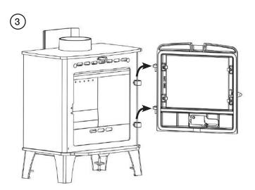
Lay the door face down on a soft flat surface, to protect the paintwork and glass.
